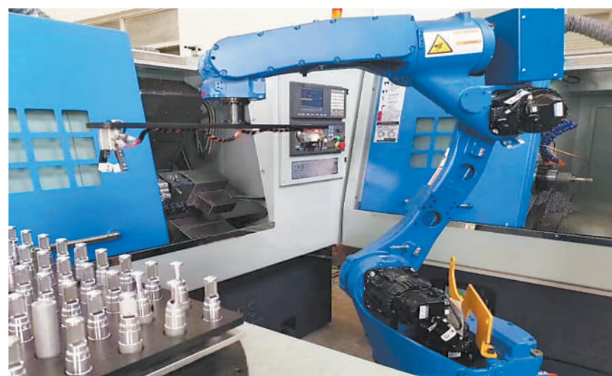
At the beginning of 2024, Zhaolv implemented a fully automated H-type automobile headlamp heat sink production line. (COURTESY PHOTO)
